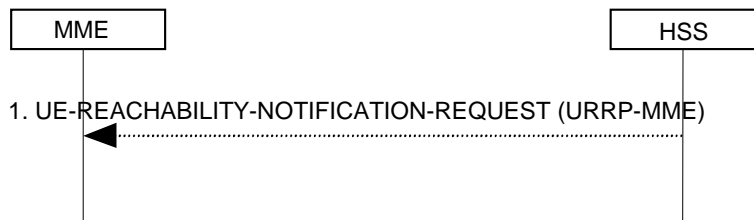
Figure 5.3.11.2-1: UE Reachability Notification Request Procedure
