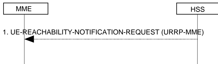
Figure 5.3.11.2-1: UE Reachability Notification Request Procedure
