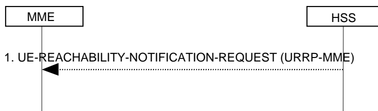
Figure 5.3.11.2-1: UE Reachability Notification Request Procedure
