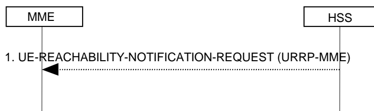
Figure 5.3.11.2-1: UE Reachability Notification Request Procedure
