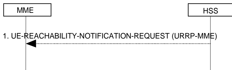
Figure 5.3.11.2-1: UE Reachability Notification Request Procedure
