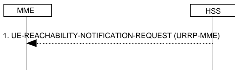
Figure 5.3.11.2-1: UE Reachability Notification Request Procedure
