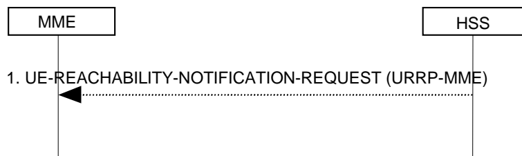
Figure 5.3.11.2-1: UE Reachability Notification Request Procedure
