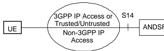
Figure 4.8.1.1-1: Architecture for Access Network Discovery Support Functions
