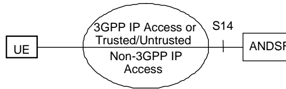
Figure 4.8.1.1-1: Architecture for Access Network Discovery Support Functions
