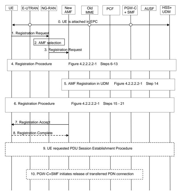
Figure 4.11.2.3-1: Mobility procedure from EPS to 5GS without N26 interface
