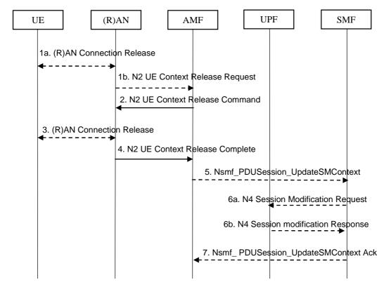
Figure 4.2.6-1: AN Release procedure
