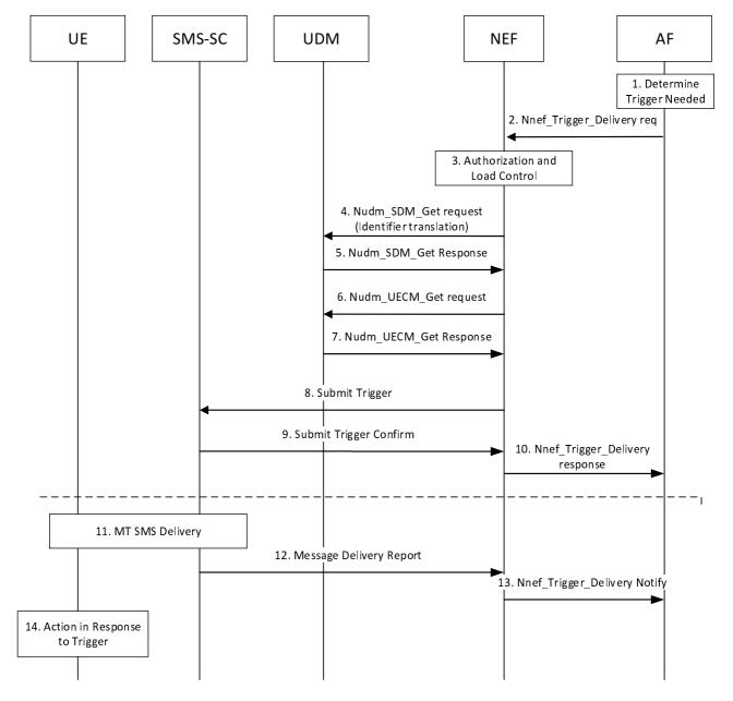
Figure 4.13.2.2-1: Device triggering procedure via Nnef
