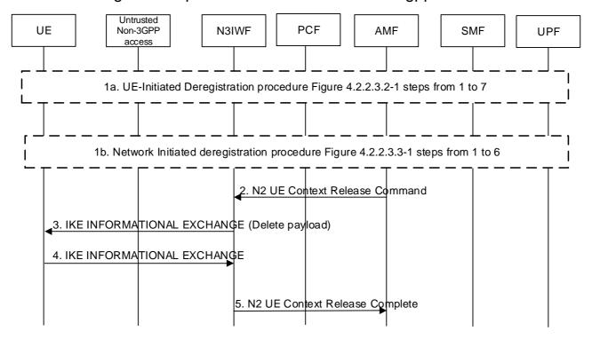
Figure 4.12.3-1: Deregistration procedure for untrusted non-3gpp access
