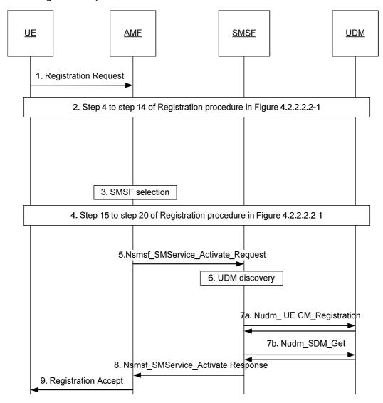
Figure 4.13.3.1-1: Registration procedure supporting SMS over NAS
