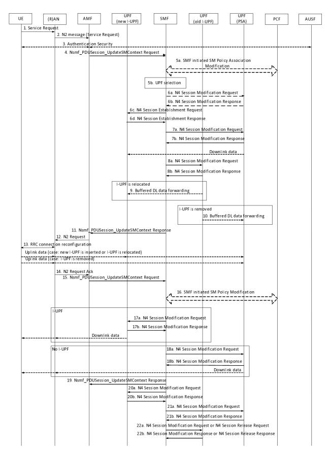
Figure 4.2.3.2-1: UE Triggered Service Request procedure
