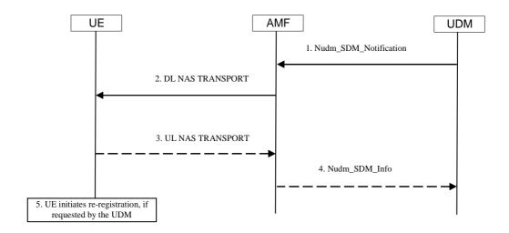
Figure 4.20.2-1: UE Parameters Update via UDM Control Plane Procedure
