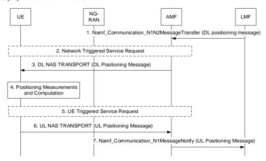
Figure 4.13.5.4-1: UE Assisted and UE Based Positioning Procedure
