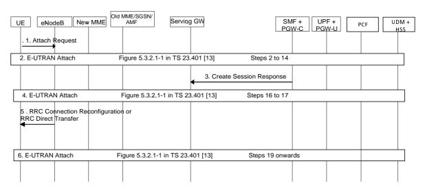
Figure 4.11.1.5.2-1: Impacts to E-UTRAN Initial Attach procedure
