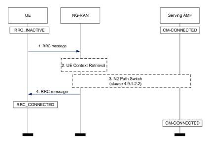
Figure 4.8.2-1: RRC Inactive to RRC Connected state transition
