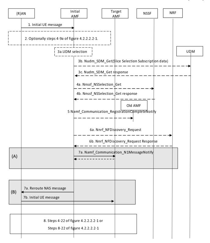
Figure 4.2.2.3-1: Registration with AMF re-allocation procedure
