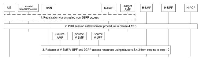
Figure 4.9.2.4.2-1: Handover of a PDU Session procedure from 3GPP access to untrusted non-3GPP access with N3IWF in the HPLMN (home routed roaming)
