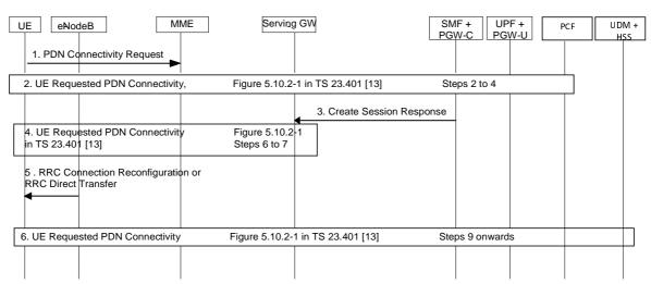
Figure 4.11.1.5.4.1-1: Impacts to UE Requested PDN Connectivity Procedure
