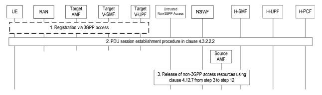
Figure 4.9.2.3.2-1: Handover of a PDU Session procedure from untrusted non-3GPP access with N3IWF in the HPLMN to 3GPP access (home routed roaming)
