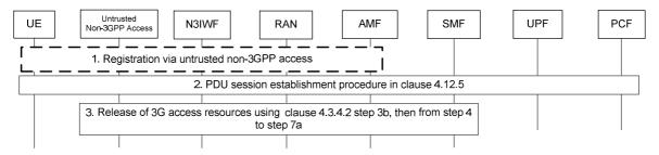
Figure 4.9.2.2-1: Handover of a PDU Session from 3GPP access to untrusted non-3GPP access (non-roaming and roaming with local breakout)
