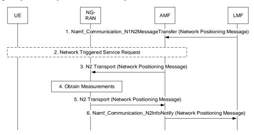
Figure 4.13.5.5-1: Network Assisted Positioning Procedure
