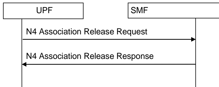
Figure 4.4.3.3-2: UPF initiated N4 association release procedure
