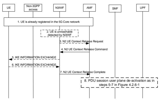
Figure 4.12.4.2-1: Procedure for the UE context release in the N3IWF
