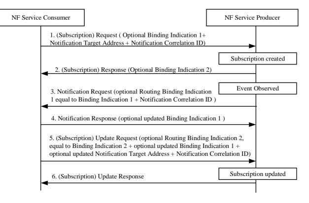
Figure 4.17.12.4-1: Binding in a subscription request
