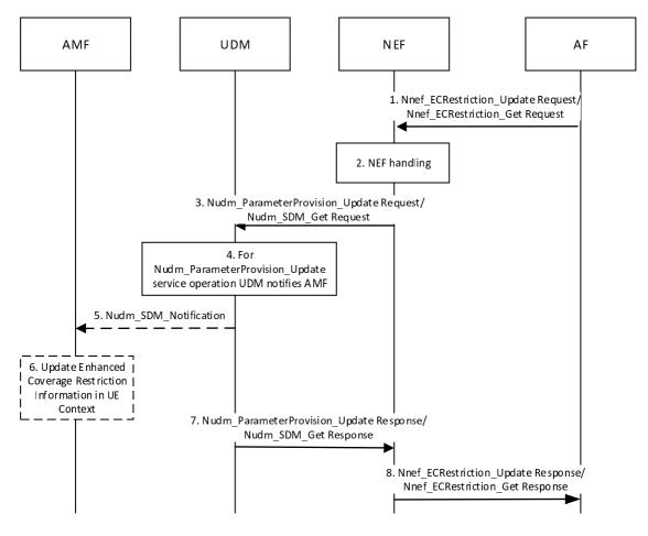
Figure 4.27.1-1: Enhanced Coverage Restriction Control via NEF
