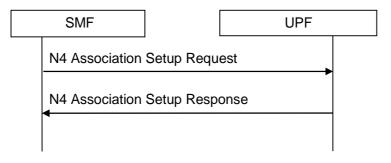
Figure 4.4.3.1-1: N4 association setup procedure initiated by SMF
