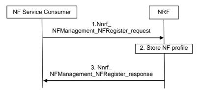
Figure 4.17.1-1: NF Service Registration procedure
