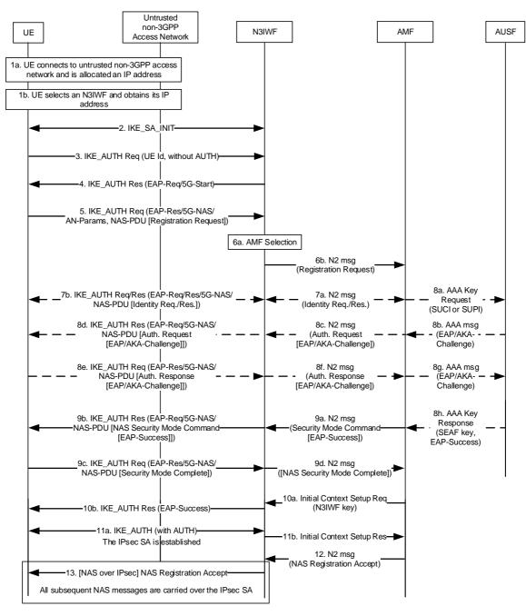
Figure 4.12.2.2-1: Registration via untrusted non-3GPP access
