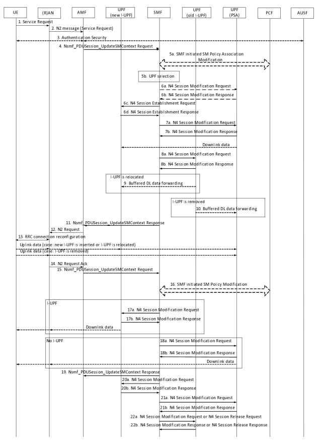
Figure 4.2.3.2-1: UE Triggered Service Request procedure
