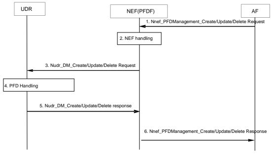
Figure 4.18.2-1 procedure for PFD management via NEF (PFDF)
