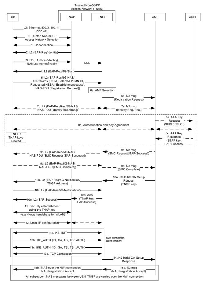
Figure 4.12a.2.2-1: Registration via trusted non-3GPP access
