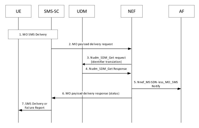
Figure 4.13.7.2-1: MSISDN-less MO SMS procedure via Nnef
