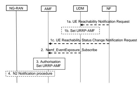
Figure 4.2.5.2-1: UE Reachability Notification Request Procedure
