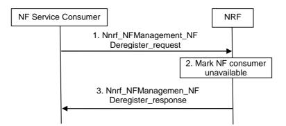
Figure 4.17.3-1: NF Service Deregistration procedure
