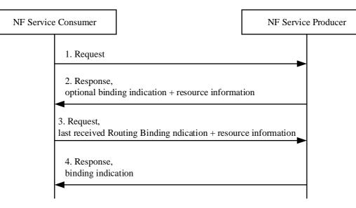
Figure 4.17.12.2-1: Binding created as part of service response
