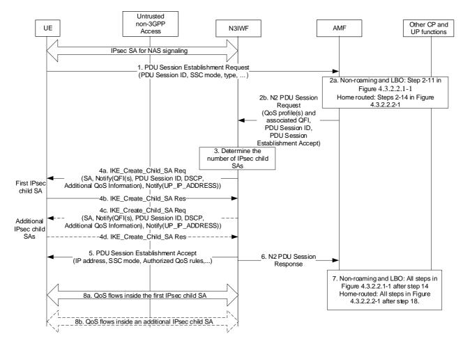
Figure 4.12.5-1: PDU Session establishment via untrusted non-3GPP access
