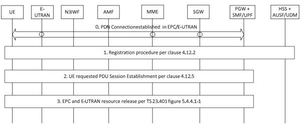
Figure 4.11.3.1-1: Handover from EPS to 5GC-N3IWF
