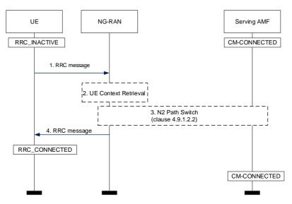
Figure 4.8.2.2-1: Connection Resume in RRC Inactive
