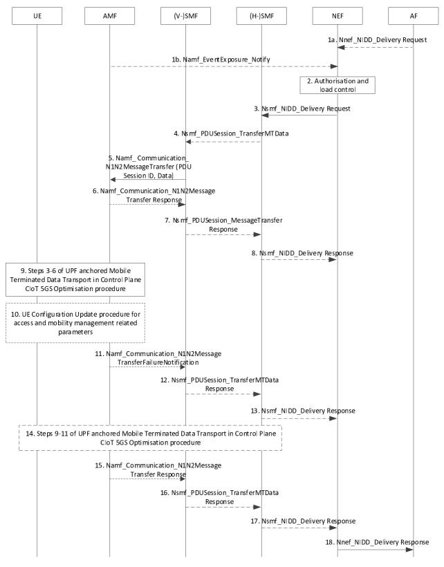
Figure 4.25.5-1: NEF Anchored Mobile Terminated Data Transport
