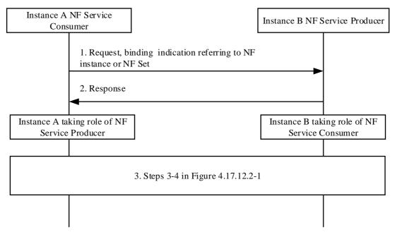
Figure 4.17.12.3-1: Binding created as part of service request
