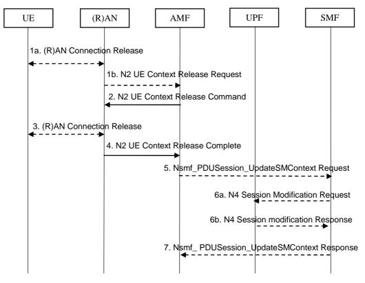
Figure 4.2.6-1: AN Release procedure
