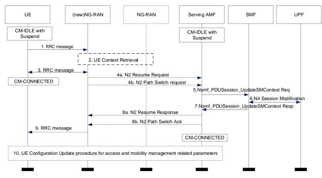
Figure 4.8.2.3-1: Connection Resume in CM-IDLE with Suspend
