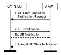
Figure 4.8.3-1: RRC state transition notification
