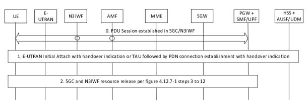
Figure 4.11.3.2-1: Handover from 5GC-N3IWF to EPS
