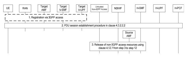
Figure 4.9.2.3.2-1: Handover of a PDU Session procedure from untrusted non-3GPP access with N3IWF in the HPLMN to 3GPP access (home routed roaming)
