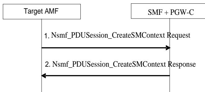
Figure 4.11.1.4.2-1: Procedures for EPS bearer IDs transfer
