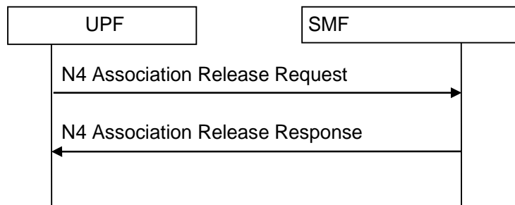
Figure 4.4.3.3-2: UPF initiated N4 association release procedure
