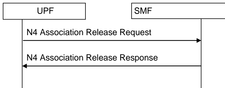
Figure 4.4.3.3-2: UPF initiated N4 association release procedure
