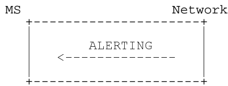
Figure 5.4/TS 24.008 Call confirmation at mobile originating call establishment
