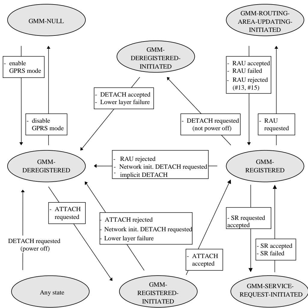
Figure 4.1b/3GPP TS 24.008:GMM main states in the MS
