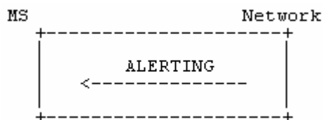
Figure 5.4/3GPP TS 24.008 Call confirmation at mobile originating call establishment
