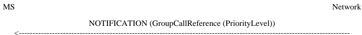
Figure 5: Signalling information between the network and the called mobile stations required for the prioritisation in case of a VGCS or VBS call
