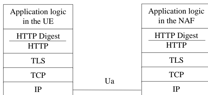
Figure 5.3.1-1: Protocol stack of Ua interface with TLS
