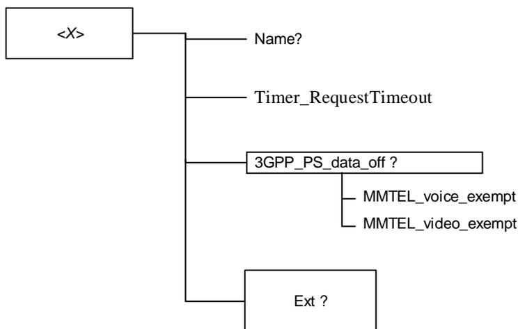
Figure 4-1: MO for BCP of MMTEL communication service
