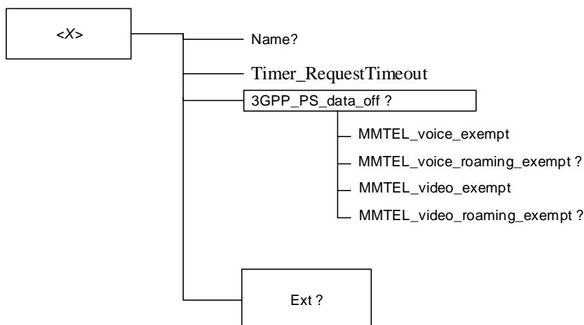
**Figure 4-1: MO for BCP of MMTEL communication service**
