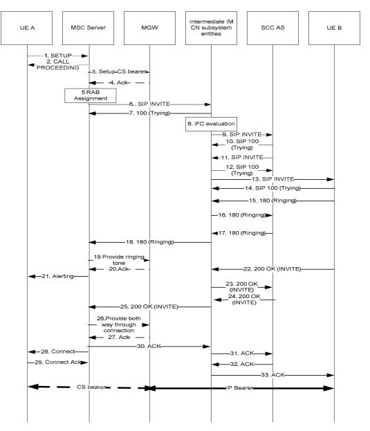
Figure A.4.4-1: CS UE Origination with CS media using an MSC Server enhanced for ICS – one codec
