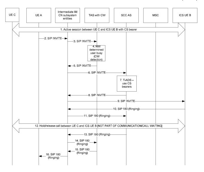
Figure A.6.3.1-1: Signalling flows for Communication Wait using Gm service control
