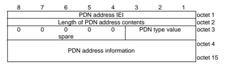
Figure 9.9.4.9.1: PDN address information element
