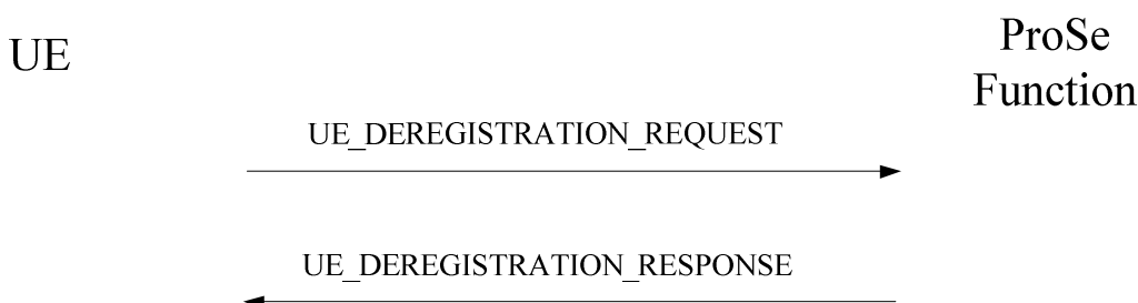
Figure 7.2.6.2.1.1: UE-initiated UE deregistration procedure
