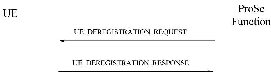
Figure 7.2.6.3.1.1: Network-initiated UE deregistration procedure
