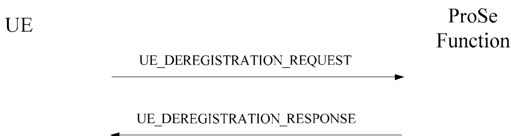
Figure 7.2.6.2.1.1: UE-initiated UE deregistration procedure
