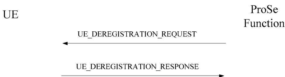
Figure 7.2.6.3.1.1: Network-initiated UE deregistration procedure
