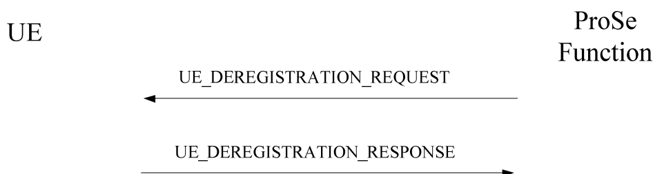
Figure 7.2.6.3.1.1: Network-initiated UE deregistration procedure
