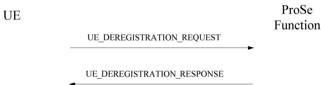
Figure 7.2.6.2.1.1: UE-initiated UE deregistration procedure
