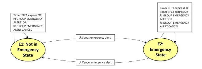
Figure 12.2.2.1: Emergency alert state machine
