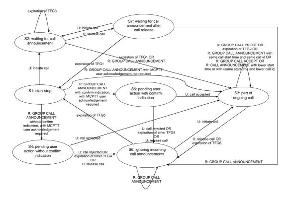
Figure 10.2.2.2-1: Basic call control state machine
