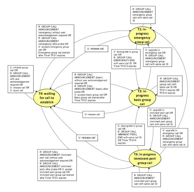
Figure 10.2.3.2-1: Call type control state machine
