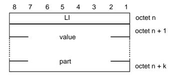
Figure I.2.2.4-7: Type 4 IE of format LV (k = 0, 1, 2, ...)
