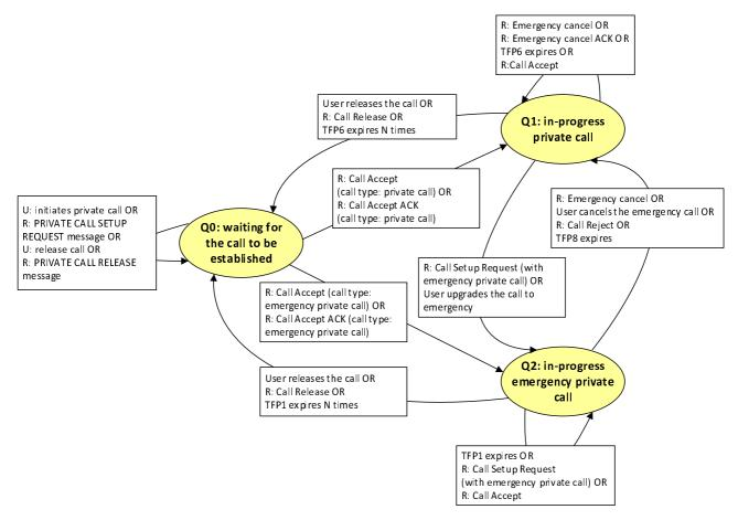
Figure 11.2.3.2-1: Call type control state machine
