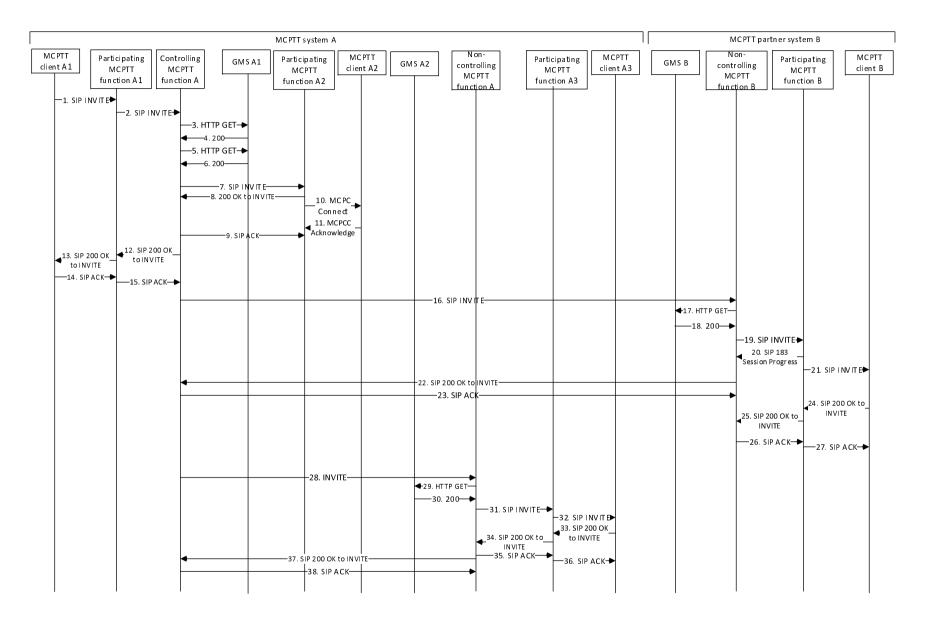
Figure A.1.3-1: Temporary prearranged group call setup
