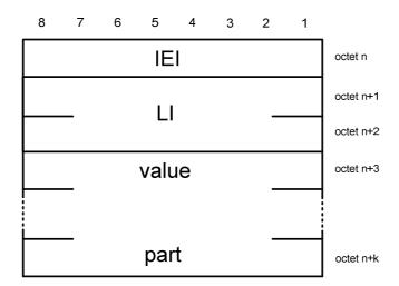
Figure I.2.2.4-10: Type 6 IE of format TLV-E (k = 1, 2, ...)
