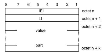
Figure I.2.2.4-8: Type 4 IE of format TLV (k = 1, 2, ...)
