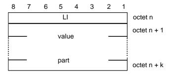
Figure I.2.2.4-7: Type 4 IE of format LV (k = 0, 1, 2, ...)
