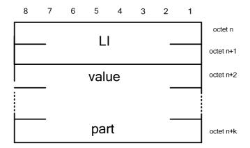
Figure I.2.2.4-9: Type 6 IE of format LV-E (k = 1, 2, ...)
