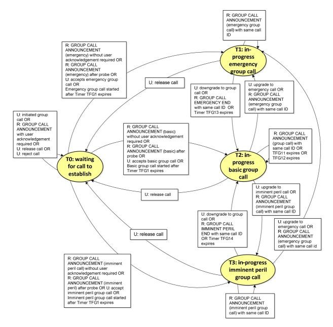
Figure 10.2.3.2-1: Call type control state machine
