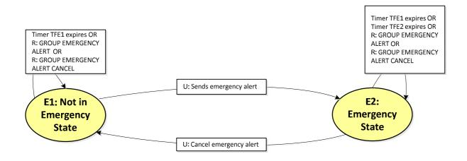
Figure 12.2.2.2-1: Emergency alert state machine
