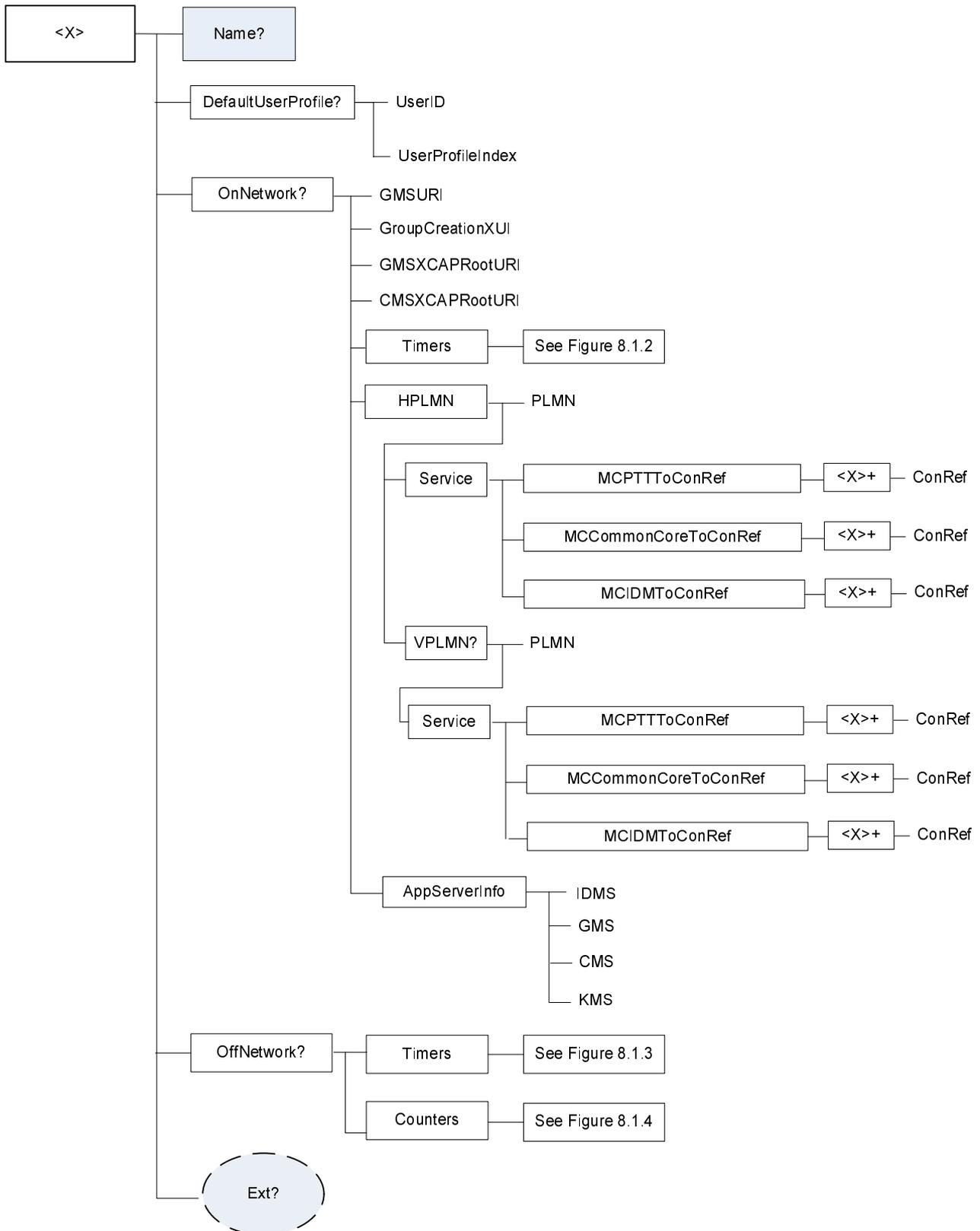
Figure 8.1.1: The MCPTT UE initial configuration MO (1 of 4)
