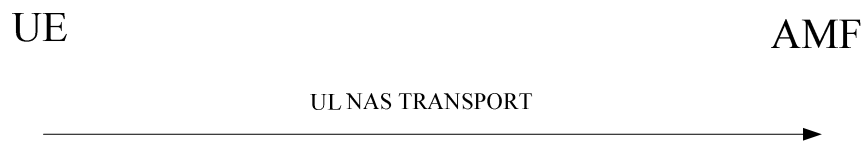
Figure 5.4.5.2.2.1: UE-initiated NAS transport procedure
