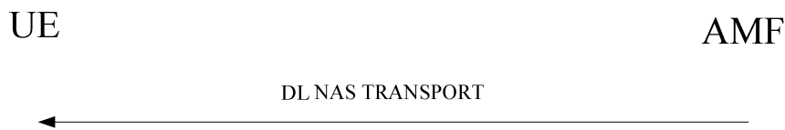
Figure 5.4.5.3.2.1: Network-initiated NAS transport procedure
