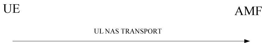
Figure 5.4.5.2.2.1: UE-initiated NAS transport procedure
