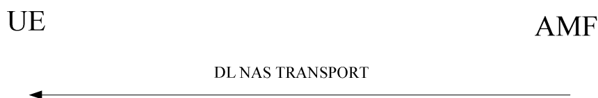
Figure 5.4.5.3.2.1: Network-initiated NAS transport procedure
