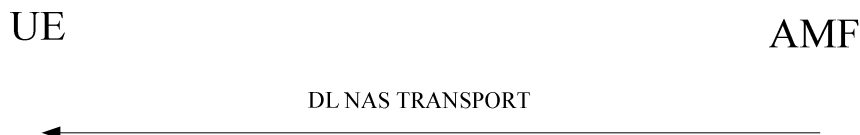
Figure 5.4.5.3.2.1: Network-initiated NAS transport procedure
