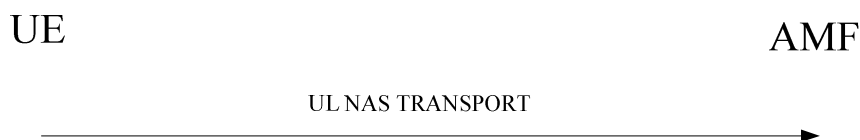
Figure 5.4.5.2.2.1: UE-initiated NAS transport procedure
