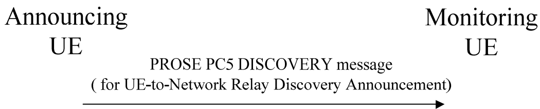
Figure 8.2.1.2.3.2.1: Monitoring UE procedure for UE-to-network relay discovery
