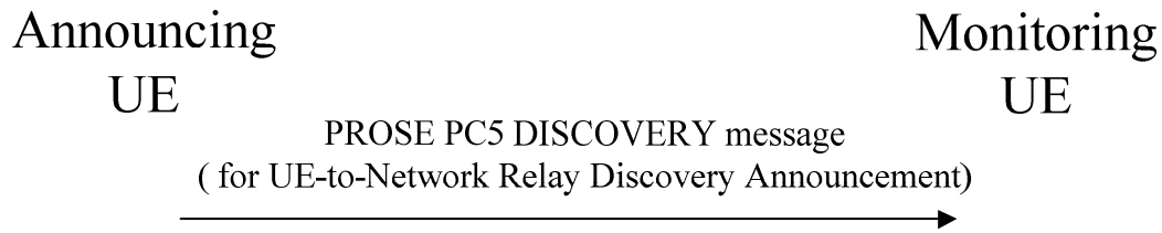
Figure 8.2.1.2.3.2.1: Monitoring UE procedure for UE-to-network relay discovery
