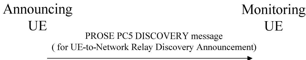
Figure 8.2.1.2.3.2.1: Monitoring UE procedure for UE-to-network relay discovery
