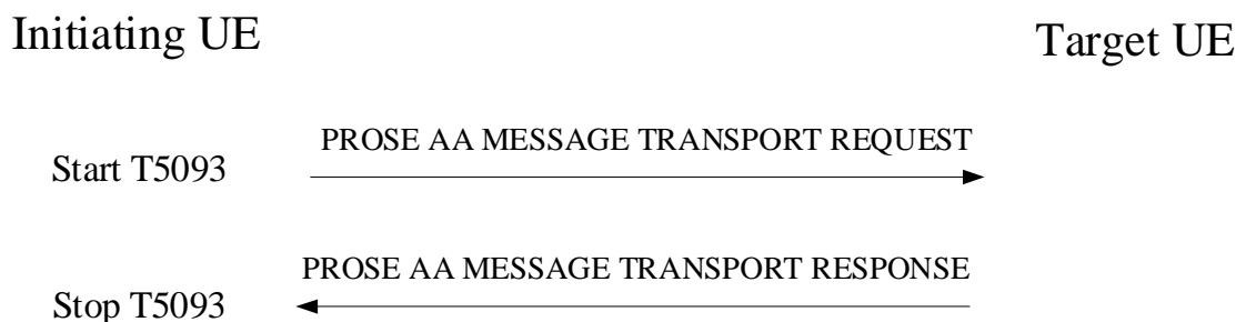
Figure 8.2.9.2.1: 5G ProSe AA message reliable transport procedure
