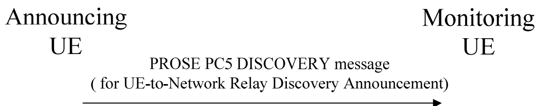
Figure 8.2.1.2.3.2.1: Monitoring UE procedure for UE-to-network relay discovery
