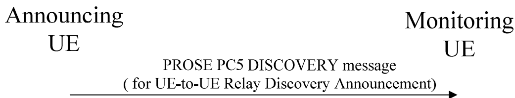
Figure 8a.2.1.2.2.2.1: Announcing UE procedure for UE-to-UE relay discovery
