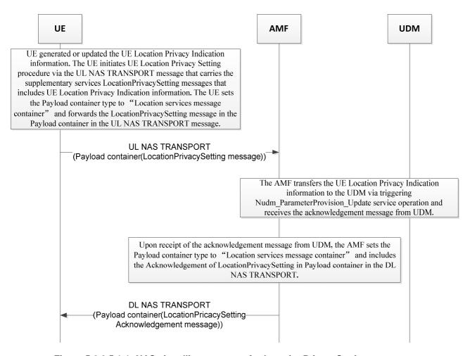
Figure 5.2.2.5.1-1: NAS signalling transport for LocationPrivacySetting messages
