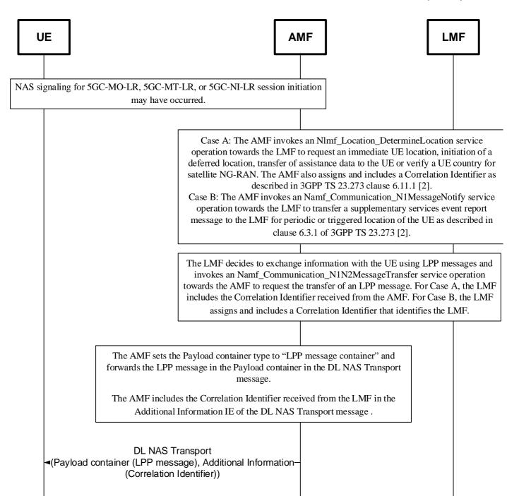
Figure 5.2.1.2.1: NAS signalling transport for downlink LPP messages
