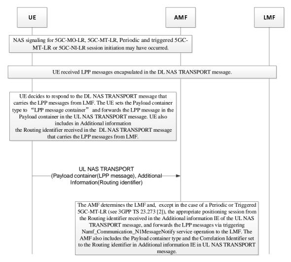
Figure 5.2.2.3-1: NAS signalling transport for uplink LPP messages
