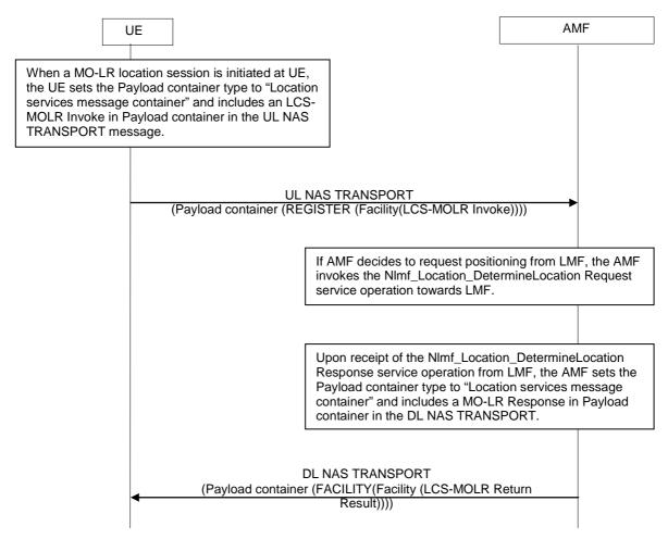
Figure 5.2.2.1.1-1: NAS signaling transport for MO-LR
