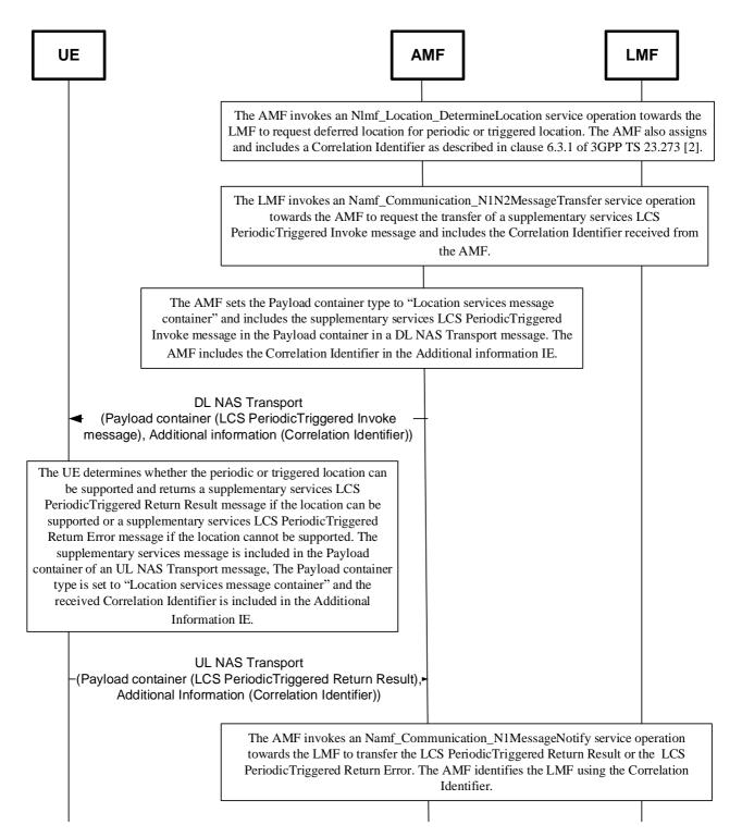
Figure 5.2.1.3.1.1: NAS signalling transport for LCS PeriodicTriggered messages
