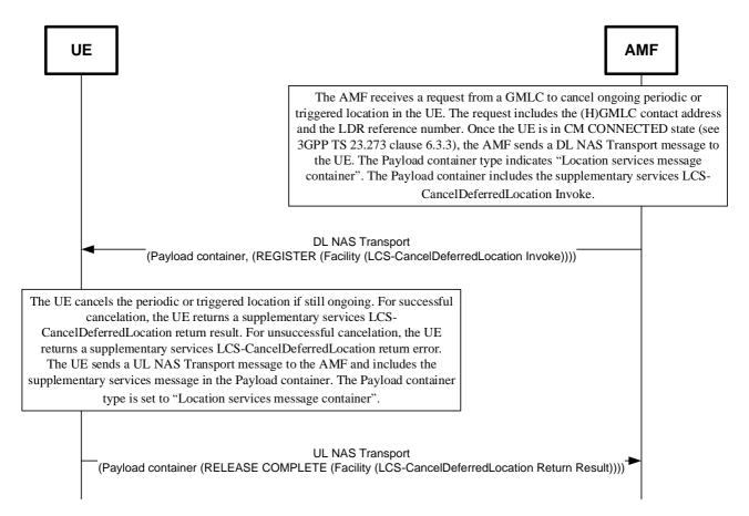
Figure 5.2.1.4.1.1: NAS signalling transport for Cancel Deferred Location
