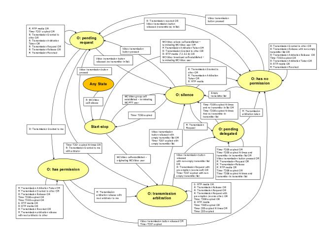
Figure 7.2.3.1-1: 'Transmission participant state diagram - basic operation'
