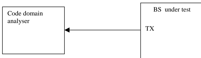
Fig.B.1 Configuration for power control steps measurement
