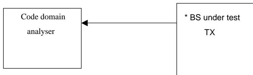
Figure B.2: Measuring system Set-up for CPICH power accuracy and peak code domain error measurements
