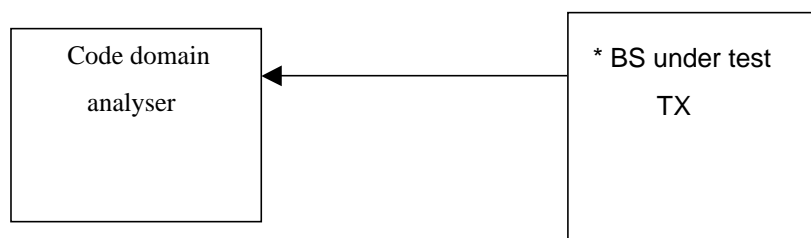
Figure B.2: Measuring system Set-up for CPICH power accuracy and peak code domain error measurements
