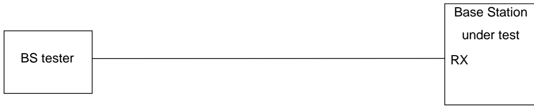
Figure B.15A: Functional Set-up for Verification of the internal BLER calculation for BS without Rx diversity
