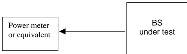
Figure B.1: Measuring system Set-up for maximum output power, total power dynamic range
