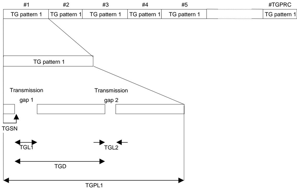
Figure 1: Illustration of compressed mode pattern parameters
