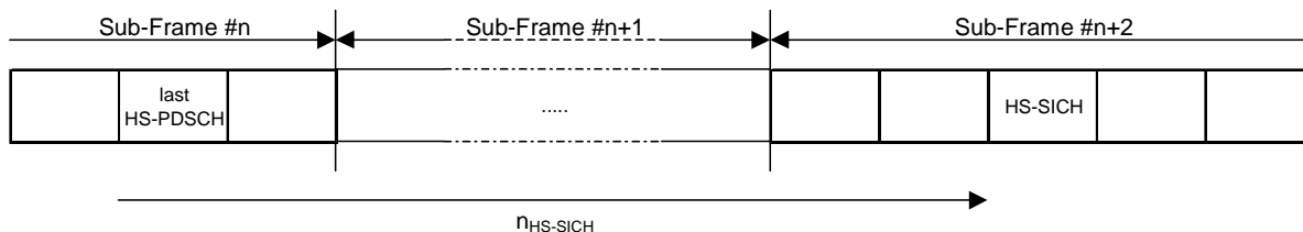
Figure 25: Timing for HS-DSCH and HS-SICH for different radio frame configurations for a given UE
