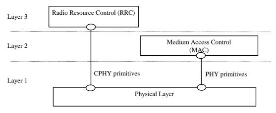
Figure 1: Interfaces with the Physical Layer
