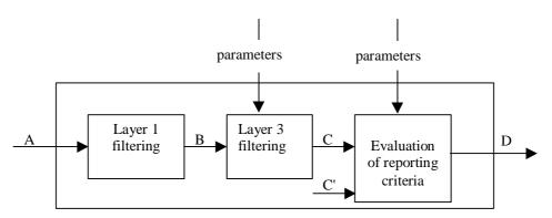
Figure 7: Measurement model
