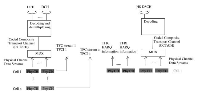
Figure 3: Model of the UE's physical layer - downlink FDD mode
