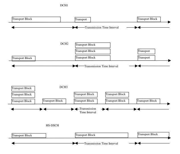
Figure 6: Exchange of data between MAC and L1
