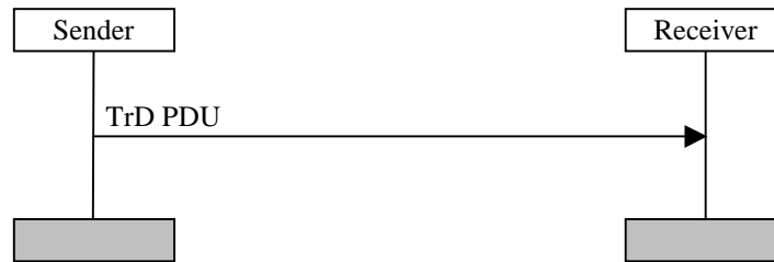
Figure 11.1: Transparent mode data transfer procedure
