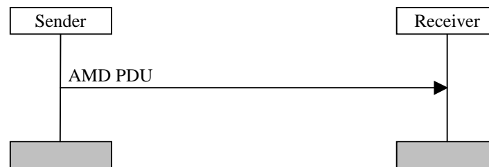
Figure 11.3: Acknowledged mode data transfer procedure
