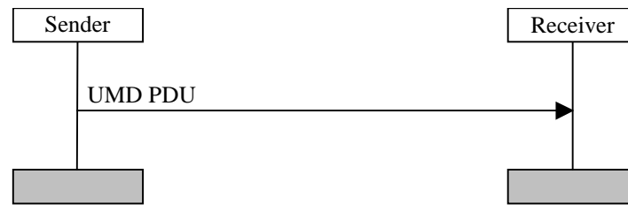
Figure 11.2: Unacknowledged mode data transfer procedure
