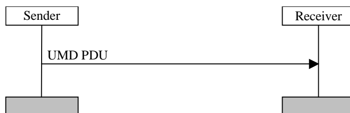
Figure 11.2: Unacknowledged mode data transfer procedure
