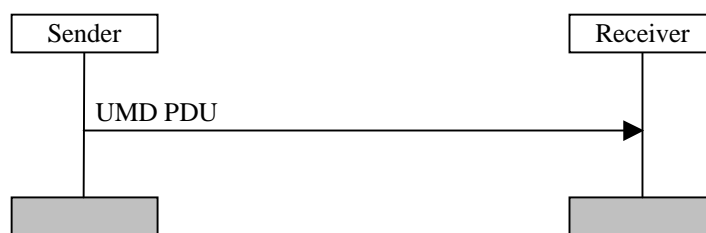
Figure 11.2: Unacknowledged mode data transfer procedure
