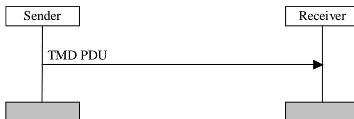
Figure 11.1: Transparent mode data transfer procedure
