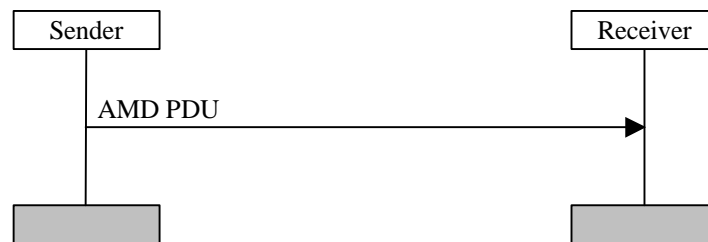
Figure 11.3: Acknowledged mode data transfer procedure
