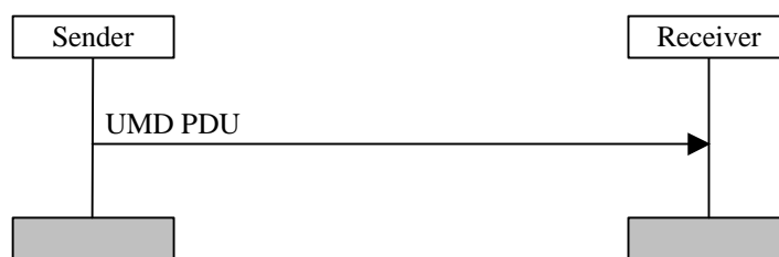
Figure 11.2: Unacknowledged mode data transfer procedure
